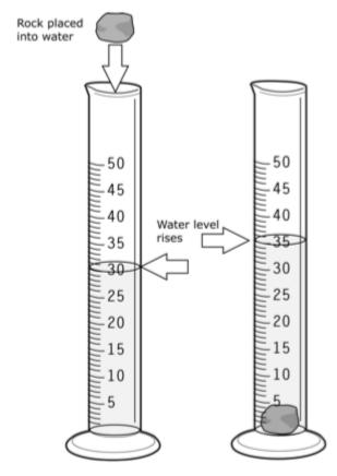
Water rose 5mL, therefore the rock has a volume of 5mL Density = mass/volume Density of rock = 15g/5mL Density = 3 g/mL
